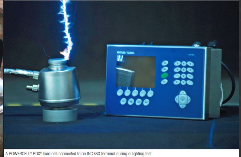
A POWERCELL® PDX® load cell connected to an iND780 terminal during a lightning test
